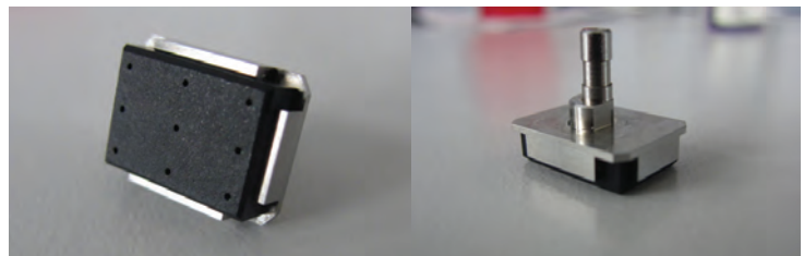
Figure 2. Left: Illustration of peeling used in the Multi Disc Ejector tool in the Die Bonder created at Besi. The pickup vacuum tool contains a rubber piece with holes for the vacuum pressure, shown at right.
